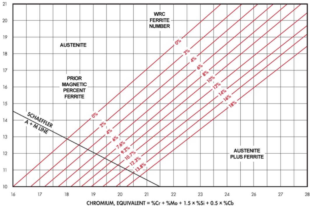
Calculate the nickel and chromium equivalents from the weld metal analysis. If nitrogen analysis of the weld is not available, assume 0.06% for GTA and covered electrode, or 0.08% for GMA weld metals. If the chemistry is accurate the diagram predicts the WRC Ferrite Number within plus or minus 3 in approximately 90% of the tests for 308, 309, 316 and 317 families.
